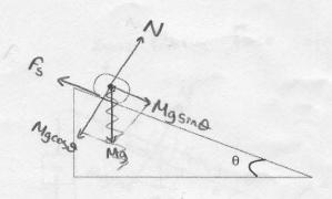
If the system is at rest, from Newton's first law:  $\Sigma f = 0$ so  $N = Mgcos\theta$  $Fs = Mgsin\theta$
